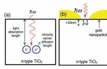
In n-type TiO2, a relatively thick film is needed to absorb a majority of the incident light, while the minority carriers (holes) recombine rapidly with the majority carriers (electrons) over a much shorter length scale. Localized plasmonic fields provide a way to mitigate this problem by coupling light very effectively from the far-field to the near-field at the metal oxide/electrolyte interface.
