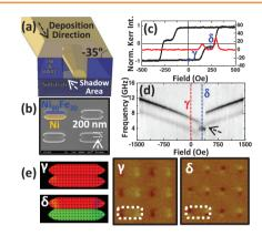
The fabrication of large area binary magnetic nanostructures made from one or two ferromagnetic materials (Ni and Ni $_{80}$ Fe $_{20}$ ) is reported using a self-aligned shadow deposition technique. Tunable magnetization switching and an adjustable dynamic response is observed for the binary structures. The results are validated by direct domain imaging using magnetic force microscopy and micromagnetic simulations.
