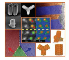
Twinning and polytypism are shown to influence the morphology of van der Waals epitaxial nanostructures. Consequently, the growth of vertically aligned nanorods and epitaxial branched crystals (tripods and tetrapods) from ZnTe can be achieved using only a single type of substrate. Crystalline characterization of the various structures is performed with extensive electron microscopy technqiues and corroborated with atomic models.
