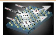
Hydrogen and deuterium atoms interact with a graphene monolayer on a Ni/Au substrate. The atoms are either adsorbed on the surface, or reflected, or they can force a previously chemisorbed atom to leave graphene in the form of a gas molecule. The kinetic isotope effect is investigated by time-dependent X-ray photoelectron spectroscopy.
